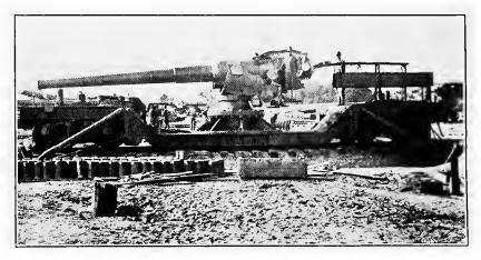
TWO VIEWS OF THE 7-INCH NAVY RIFLE MOUNTED ON A PEDESTAL ON A RAILWAY CAR.
