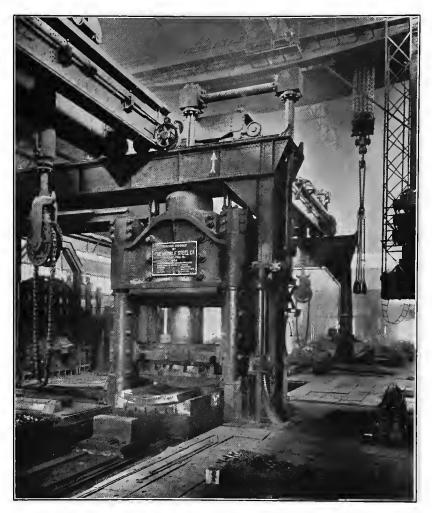
A 9,000-TON HYDRAULIC FORGING PRESS IN THE PLANT OF THE MIDVALE STEEL CO.
