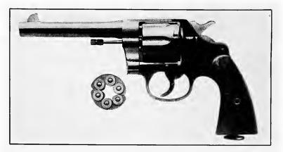
COLT DOUBLE ACTION REVOLVER, CALIBER .45, MODEL 1917.
