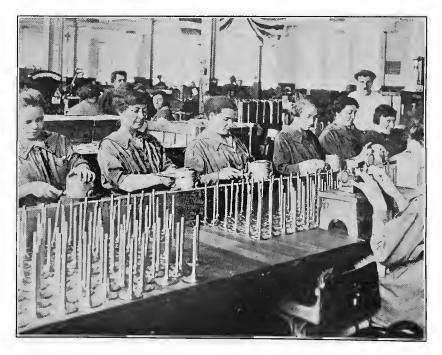
GAUGING VALVES AND PISTONS FOR THE LIBERTY ENGINE. LINCOLN MOTOR CO.
