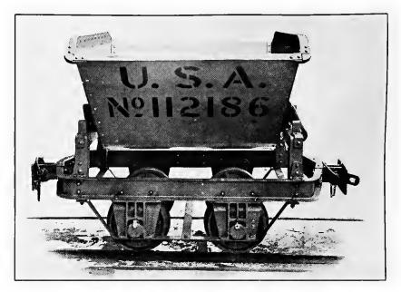
60-CENTIMETER GAUGE V-SHAPED DUMP CARS. Capacity, 27 cubic feet. Length over couplers, 6 feet 9 inches. Width of body, 48% inches.
